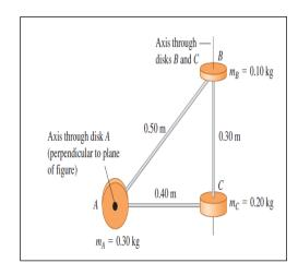
The moment of inertia about axis *A* is greater than that about axis *BC*. Hence of the two axes it's easier to make the machine part rotate about axis *BC*.
