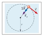
**Ex**: A puck of mass 0.5 kg is attached to the end of a cord 1.5 m long. The puck moves in a horizontal circle. If the cord can withstand a maximum tension of 50 N, what is the maximum speed at which the puck can move before the cord breaks? Assume the string remains horizontal during the motion.
