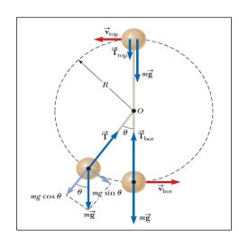
**Ex**: A 0.15 kg ball on the end of a 1.1 m long cord (negligible mass) is swung in a vertical circle. (*a*) Determine the minimum speed the ball must have at the top of its arc so that the ball continues moving in a circle. (*b*) Calculate the tension in the cord at the bottom of the arc, assuming the ball is moving at twice the speed of part (*a*).
