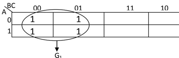
$$\begin{aligned} F &= G_1 \\ &= \overline{B} \end{aligned}$$
