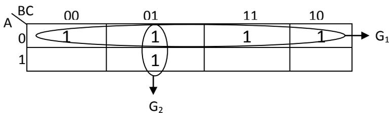
$$\begin{aligned} F &= G_1 + G_2 \\ &= \overline{A} + \overline{B}C \end{aligned}$$
