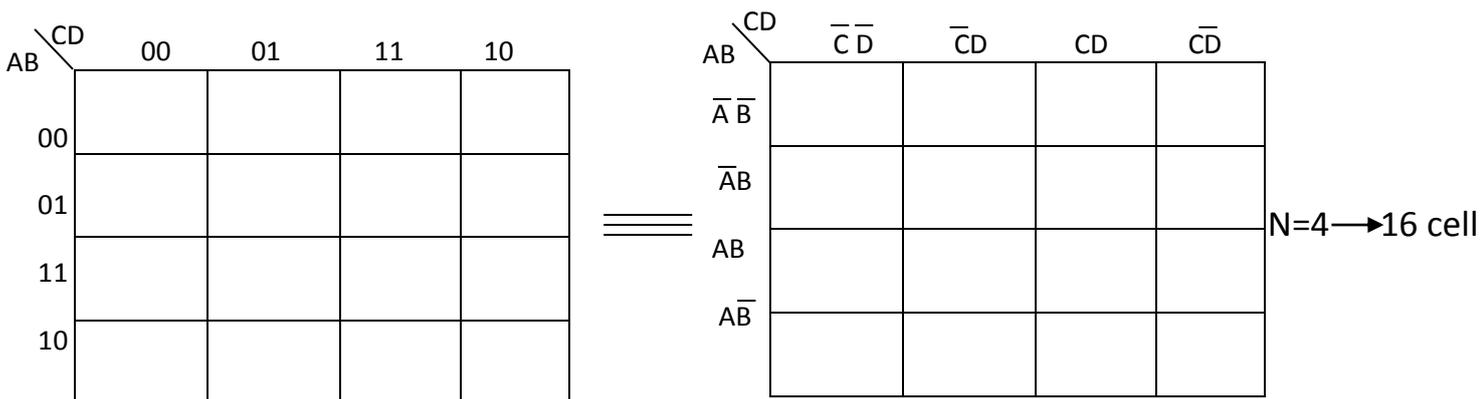
The first step in the minimization method is to implement the T.T. to the K-map. 1's and 0's in the output of the T.T. is placed in the cells corresponding to the input variables of the T.T.
