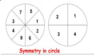
Circle sections in adjacent octants within one quadrant are symmetric with respect to the 45' line dividing the two octants.
