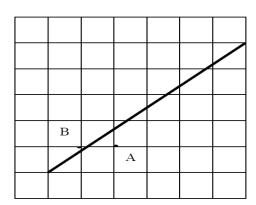
Although it may not be possible to choose pixels that lie on the actual line, we want to turn on pixels lying closest to it. For example, in previous figure, the pixel at location B is a better choice than the one at location A.
