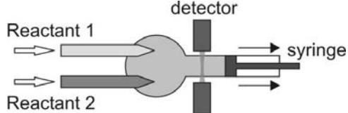
All flow techniques share the common problem that contributions from heterogeneous reactions at the walls of the flow tube can complicate the experiments. These can be minimised by coating the inner surface of the flow tube with an unreactive substance such as teflon or halocarbon wax, and the relative contributions from the process under study and reactions involving the walls may be quantified by varying the diameter of the flow tube (and therefore the ratio of volume to surface area).
