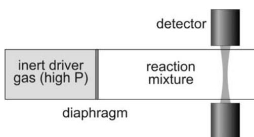
essentially consists of two chambers separated by a diaphragm. One chamber contains the appropriate mixture of reactants and precursor, the second an inert gas at high pressure. To initiate reaction, the diaphragm is punctured and a shock wave propagates through the reaction mixture. The temperature rise can be controlled by varying the pressure and composition of the inert gas. The composition of the reaction mixture after initiation is monitored in real time, usually spectroscopically.
