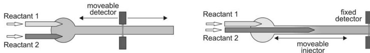
Continuous flow methods have the disadvantages that relatively large quantities of reactants are needed, and very high flow velocities are required in order to study fast reactions. These problems may be avoided by using a *stopped flow technique*. In this method, a fixed volume of reactants are rapidly flowed into a reaction chamber and mixed by the action of a syringe fitted with an end stop
