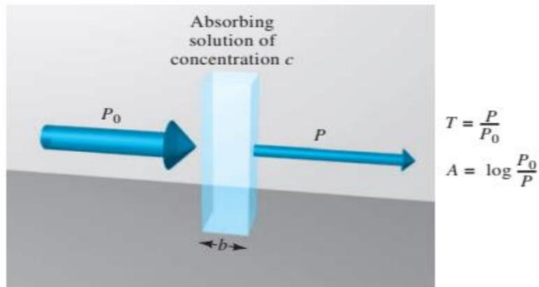
Attenuation of a beam of radiation by an absorbing solution. The larger arrow on the incident beam signifies a higher radiant power  $P^0$  than that transmitted by the solution  $P$ . The path length of the absorbing solution is  $b$  and the concentration is  $c$ .
