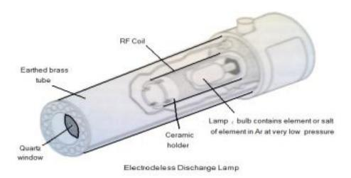
How does an EDL lamp work? When the ceramic cylinder is heated, the bulb containing the metal salt is heated and the metal is heated as a result of heating the ceramic container and the salt CaCl2 decomposes into Ca and Cl and excited atoms emerge after absorbing energy. The calcium atom Ca absorbs energy and is excited into \*Ca and when it returns to its original state, i.e. losing energy, it emits a RR $\lambda$
