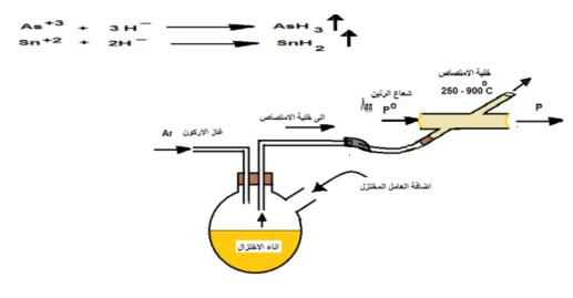
In the absorption cell, due to the presence of a high temperature, the positive ions of these hydrides are transformed into free, neutral atoms that have the ability to absorb their resonance beam that passes through the absorption cell.
