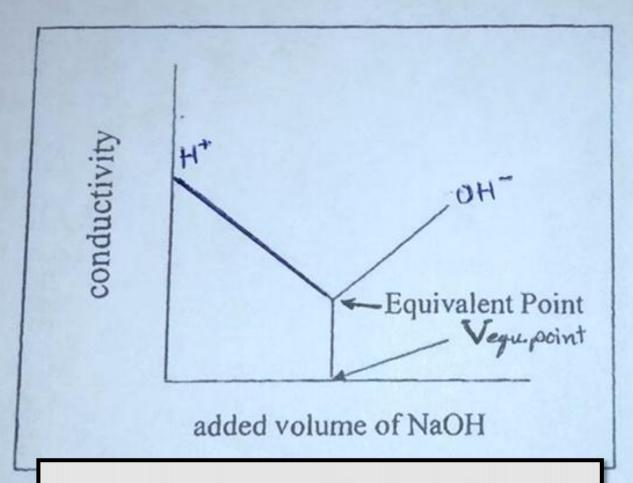
$$(N \times V)_{HCI} = (N \times V)_{NaOH}$$
