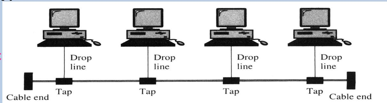
As a **signal** travels along the backbone, **some of its energy is transformed into heat**. Therefore, it **becomes weaker and weaker as it travels farther and farther**. For this reason there is a limit on the number of taps a bus can support and on the distance between those taps.
