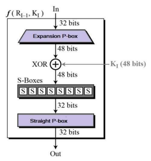
**Expansion Permutation Box** – Since right input is 32-bit and round key is a 48-bit, we first need to expand right input to 48 bits. Permutation logic is graphically depicted in the following illustration –
