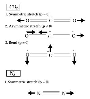
Figure 7-10 Normal vibrational modes of  $CO_2$  and  $N_2$
