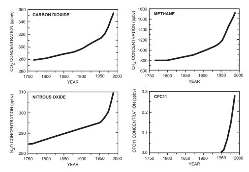
Figure 7-1 Rise in the concentrations of greenhouse gases since the 18th century
