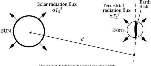
Figure 7-9 Radiative balance for the Earth
