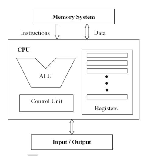
The CPU fetches instructions from memory, reads and writes data from and to memory, and transfers data from and to input/output devices. A typical and simple execution cycle can be summarized as follows:
