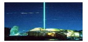
Light Detection and Ranging (LIDAR) is an ozone measurement technique that relies on absorption of laser light by ozone. A telescope is used to collect ultraviolet light that is scattered by two laser beams - one of which is absorbed by ozone (308 nm) and the other is not (351 nm). By comparing the intensity of light scattered from each laser, a profile of ozone concentration vs. altitude is measured from 10 km to 50 km.
