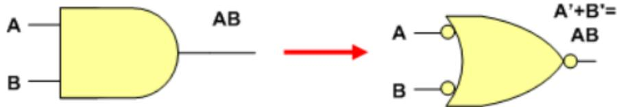
A NOR gate is equivalent to an inverted-input AND gate.
