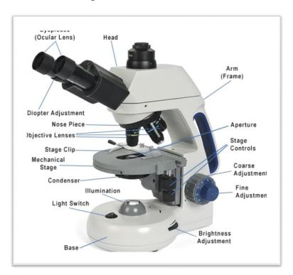
Figure 1-2 show binocular Compound microscope
