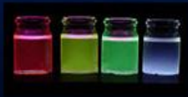
Solutions of differently sized CdSe quantum dots
