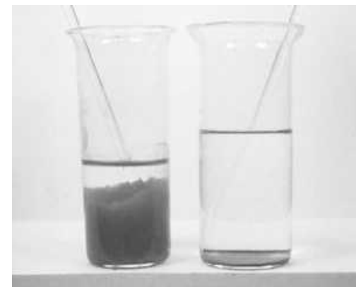
Figure: Aluminum hydroxide formed by the direct addition of ammonia (left) and the homogeneous production of hydroxide (right).
