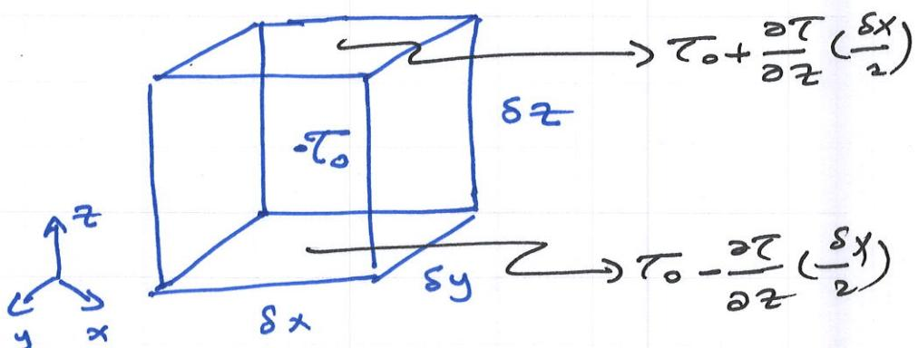
on the bottom face of the cube, the force in the  $x$ -direction is:  $\tau_0 - \frac{\partial \tau}{\partial z} \left( \frac{\delta x}{2} \right)$
