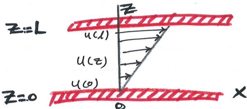
The layer in contact with the upper and lower plates will move as the following:
