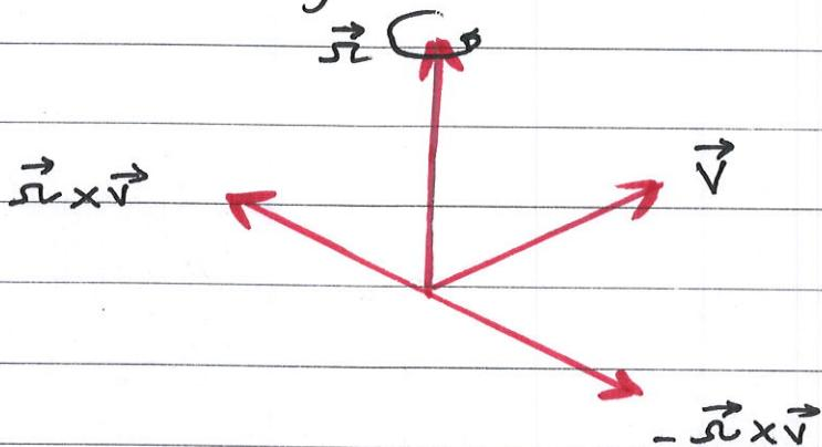
In the northern hemisphere, where  $\omega$  is counterclockwise, the Coriolis force acts to the right of the velocity vector, it tends to deflect air parcel to the right of their direction of motion.
