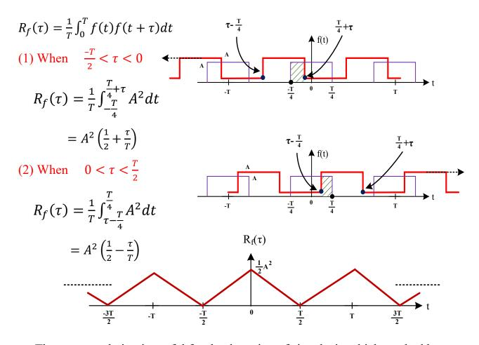
The autocorrelation is useful for the detection of signals, in which masked by additive noise, see the following figures.
