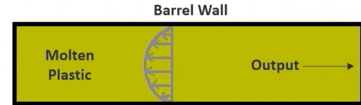
Velocity flow profile of pressure flow
