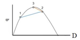
Slope of line 2-3 is the velocity of shockwave after exit of the truck (the flow is at the capacity)
