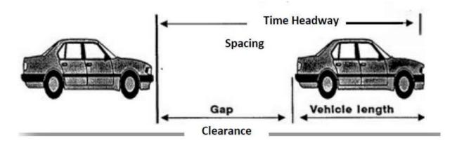
It can be computed as the difference between the time the front of a vehicle arrives at a point on the highway  $(t_1)$  and the time the front of the next vehicle arrives at the same point  $(t_2)$ . It is usually expressed in seconds.
