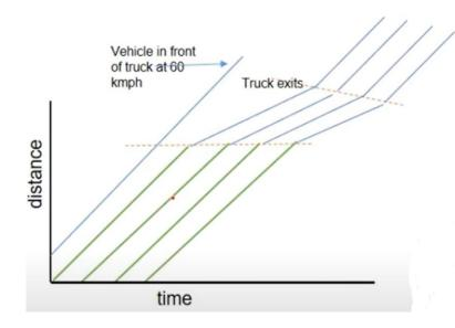
State 1 – free flow State 2 – platooning behind a slow truck State 3 – flow with full capacity
