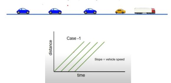
b. A truck moving at a low speed (for example 20km/hr), and the passing is not permitted, then all vehicle which are following the truck will be forced to travel at the same speed. A plateau will be formed behind the truck and this platoon will be moving at the same speed.
