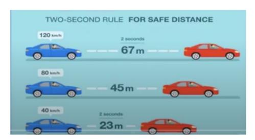
The average time headway in a lane is directly related to the rate of flow:
