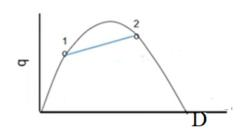
**Slope of line 1-2** is the velocity of shockwave.
