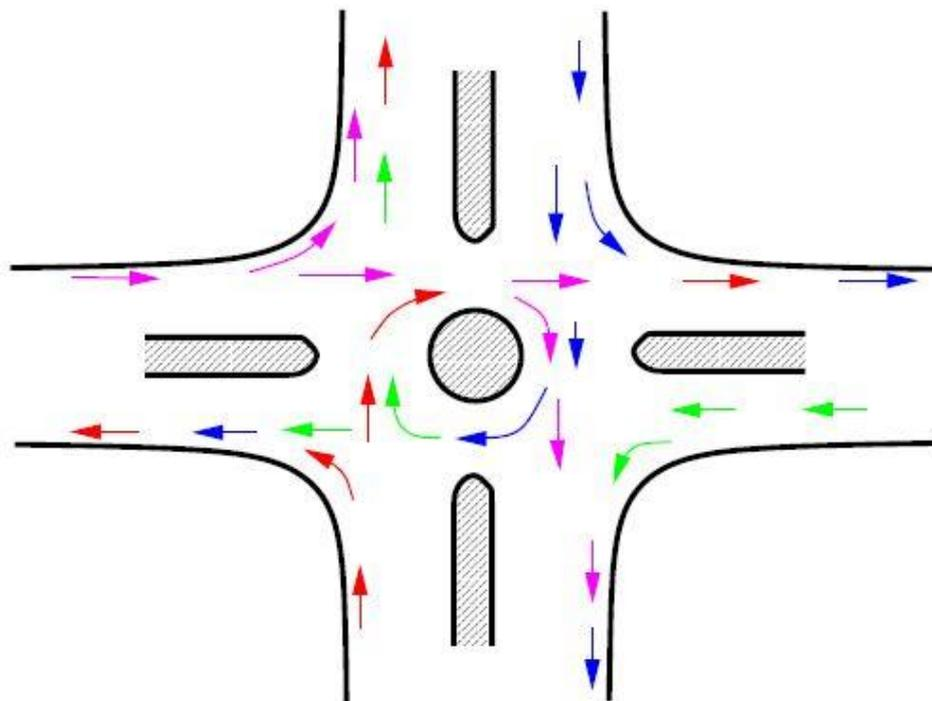
**Figure: Channelization of Traffic through a Four-legged Intersection.**
