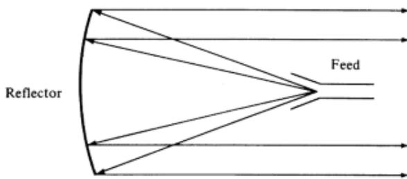
parabolic reflector with front feed
