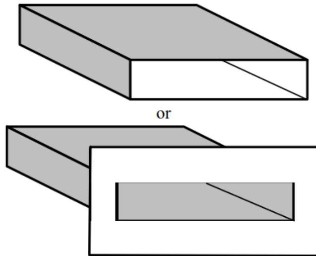
(c) open rectangular waveguide
