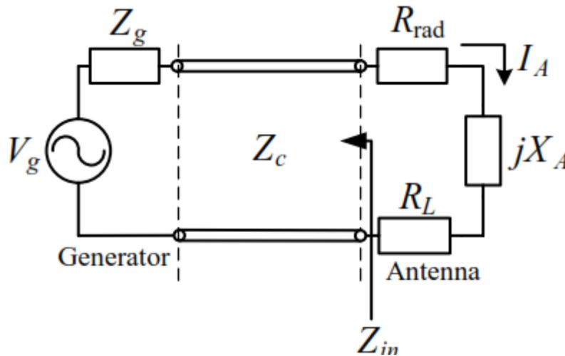
$V_g$  - voltage-source generator (transmitter);
