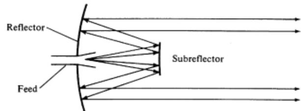
Parabolic reflector with cassegrain feed
