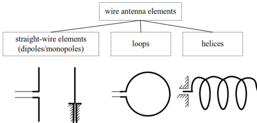
Wire antennas are simple to make but their dimensions are commensurable with the wavelength. This limits the frequency range of their applicability (at most 1-2 GHz). At low frequencies, these antennas become increasingly large.
