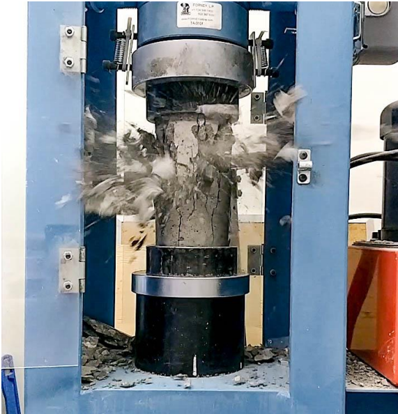
Compressive strength test
