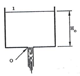
Applying Bernoulli's theorem between the surface of the water 1 and the orifice 0 yields
