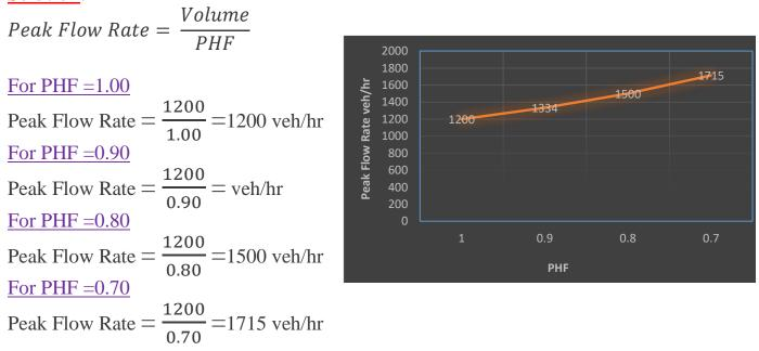
Low values of PHF illustrated that there is significant variation of traffic volume within the peak hour volume and higher values of PHF means the traffic volume is approximately equal within peak hour period.
