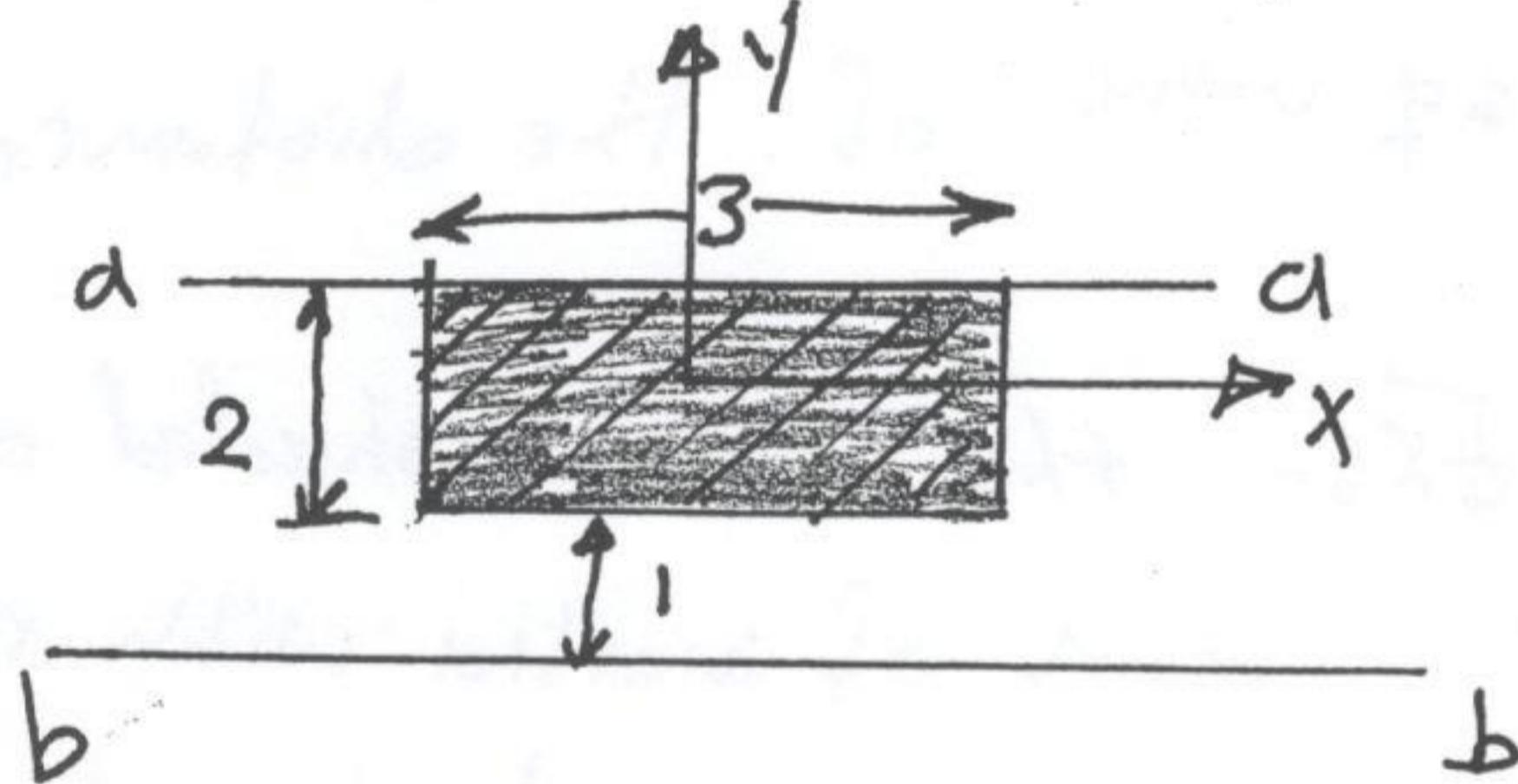
6.2 The area is  $10 \text{ cm}^2$ ,  $J_c = 30 \text{ cm}^4$ ,  $I_d = 22 \text{ cm}^4$ . Determine the mom. of inertia with respect to b-axis.
