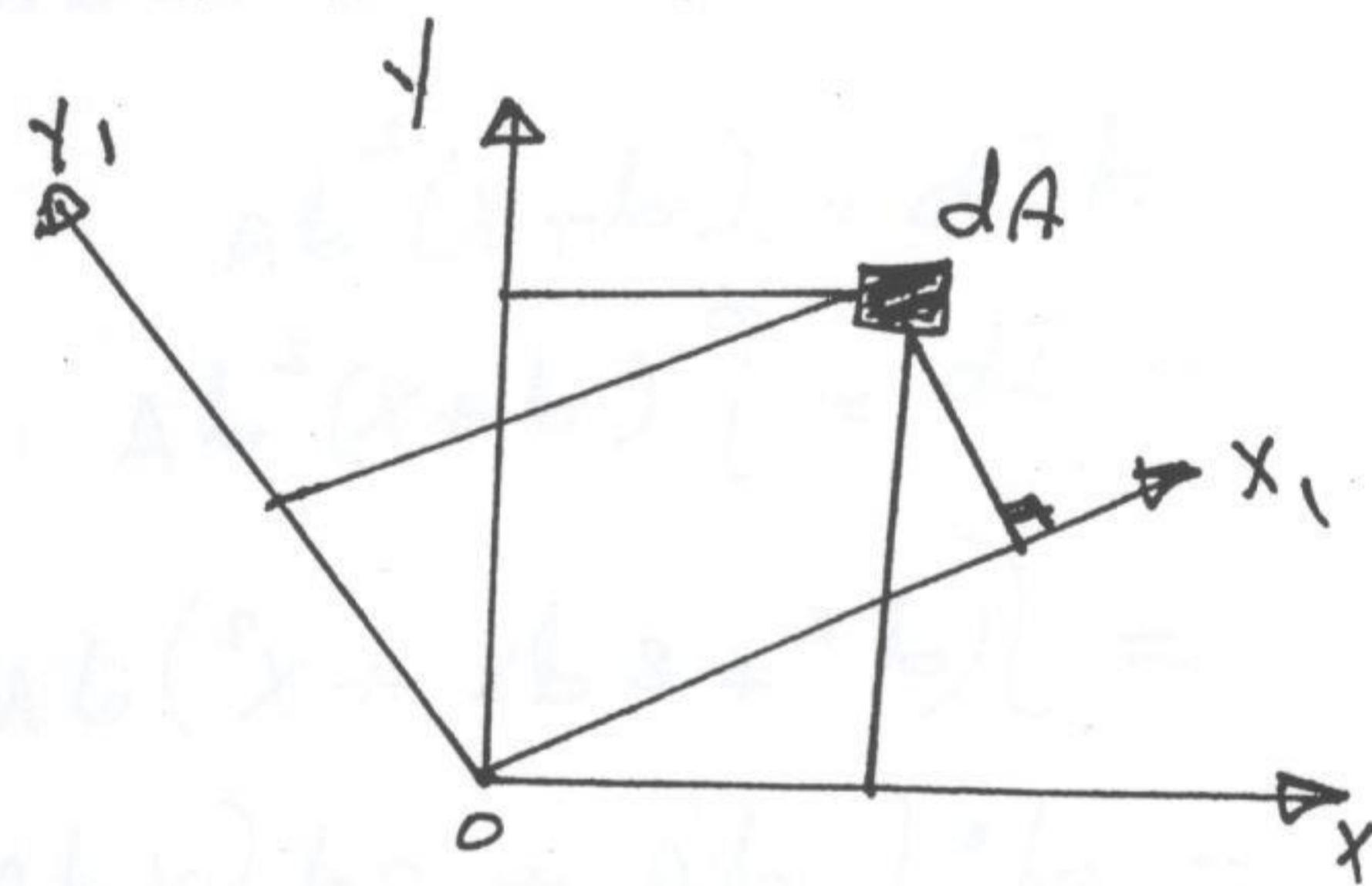
The moment of inertia of an area is always positive and has dimensions of (length) ( $m^4$ ,  $mm^4$ ,  $cm^4$ )
