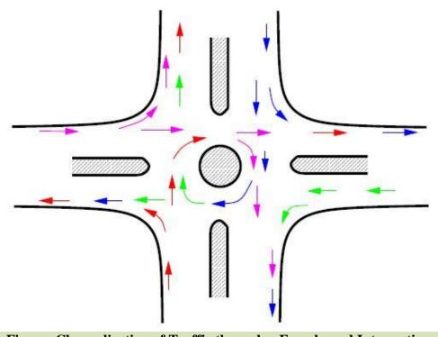
Figure: Channelization of Traffic through a Four-legged Intersection.
