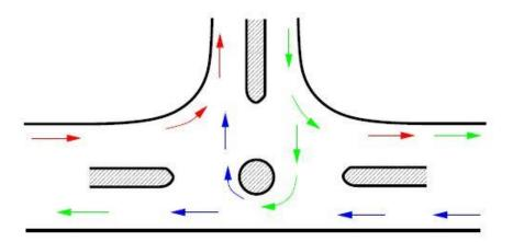
Figure: Channelization of Traffic through a Three-Legged Intersection.
