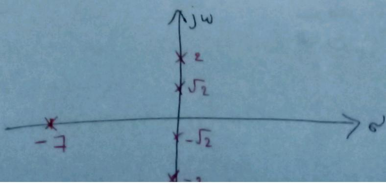
Ex 4: Find the range  $K$ , for the system shown below that will cause the system to be stable, unstable and marginally stable. Find also the value of freq. For marginally stable. Assume  $K > 0$
