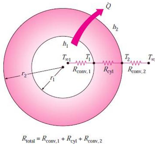
Figure 2-13 The thermal resistance network for a cylindrical (or spherical) shell subjected to convection from both the inner and the outer sides
