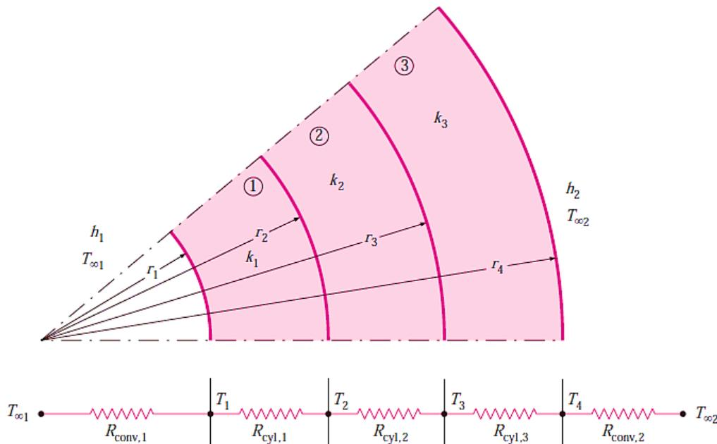
Figure 2-14 The thermal resistance network for heat transfer through a three-layered composite cylinder subjected to convection on both sides
