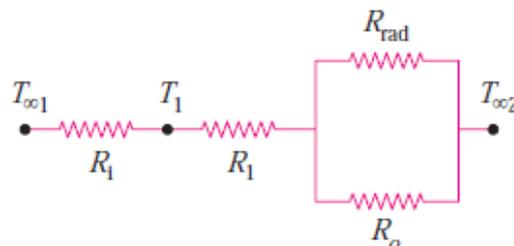
The thermal resistance network for this problem is given in figure 2–15. Noting that the inner diameter of the tank is  $D_1 = 3 \text{ m}$  and the outer diameter is  $D_2 = 3.04 \text{ m}$ , the inner and the outer surface areas of the tank are
