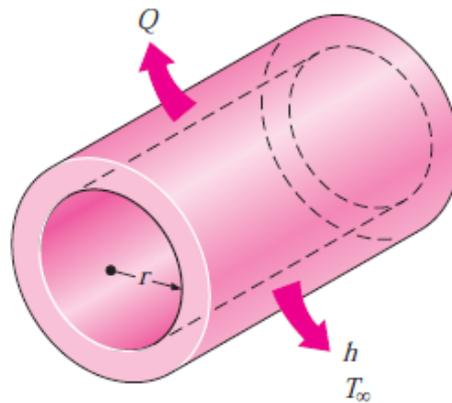
Figure 2-11 Heat is lost from a hot-water pipe to the air outside in the radial direction, and thus heat transfer from a long pipe is one-dimensional
