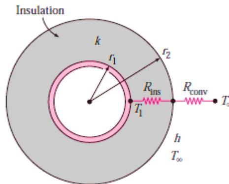
Figure 2-16 An insulated cylindrical pipe exposed to convection from the outer surface and the thermal resistance network associated with it.
