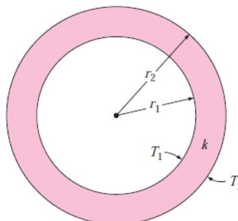
Figure 2-12 A long cylindrical pipe (or spherical shell) with specified inner and outer surface temperatures  $T_1$  and  $T_2$ .
