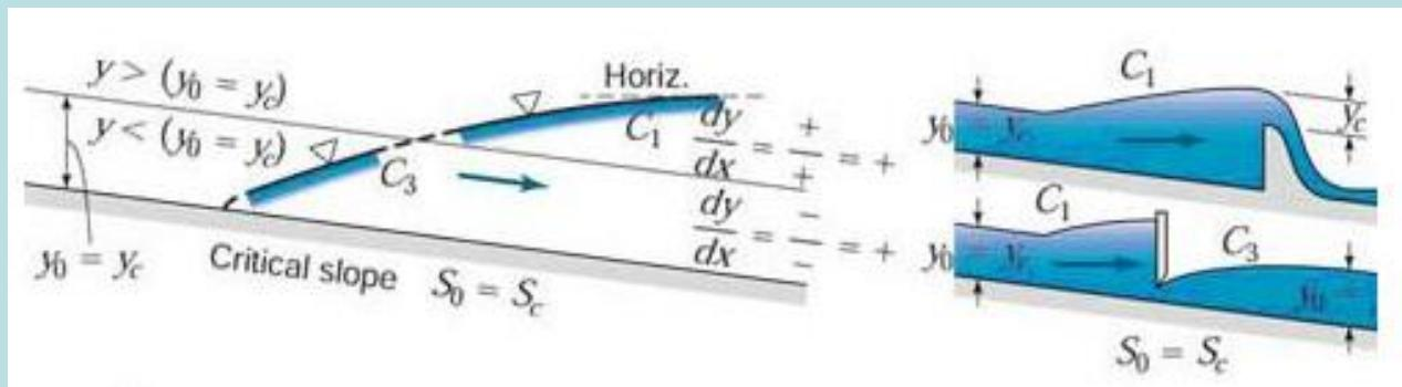
$$\frac{dh}{dx} = S_f - \frac{\frac{1}{2} \left( \frac{q^2}{h^3 C^2 S_f} \right)}{1 - \frac{q^2}{gh^3}} = S_f \frac{1 - \left( \frac{h_n}{h} \right)^{10/3}}{1 - \left( \frac{h_c}{h} \right)^3}$$
