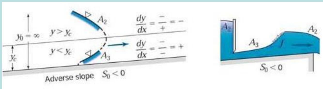
$$\frac{dh}{dx} = S_f \frac{1 - \left( \frac{q^2}{h^3 C^2 S_f} \right)}{1 - \frac{q^2}{gh^3}} = S_f \frac{1 - \left( \frac{h_n}{h} \right)^{10/3}}{1 - \left( \frac{h_c}{h} \right)^3}$$
