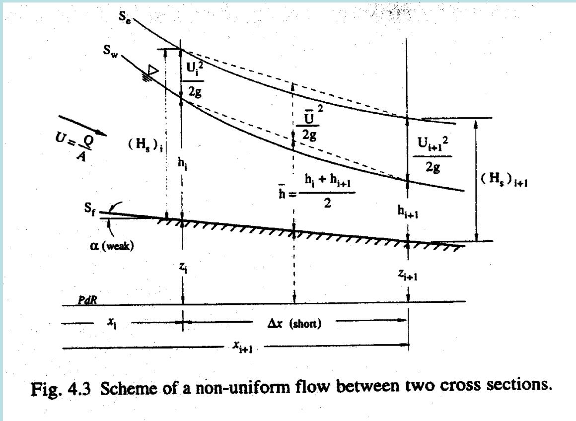
Fig. 4.3 Scheme of a non-uniform flow between two cross sections.
