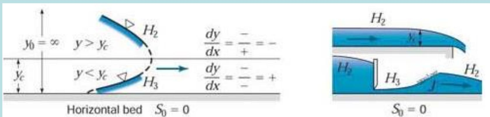
$$\frac{dh}{dx} = S_f \frac{1 - \left( \frac{q^2}{h^3 C^2 S_f} \right)}{1 - \frac{q^2}{gh^3}} = S_f \frac{1 - \left( \frac{h_n}{h} \right)^{10/3}}{1 - \left( \frac{h_c}{h} \right)^3}$$
