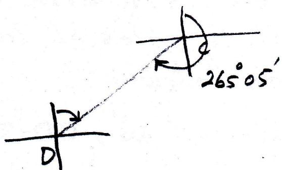
$$\begin{aligned}\text{Forward } CD &= 265^\circ 05' \\ \text{backward } CD &= 265^\circ 05' - 180^\circ \\ &= 85^\circ 05'\end{aligned}$$
