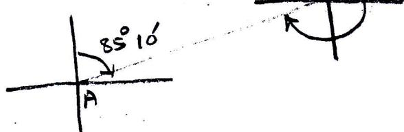
$$\begin{aligned} \text{Forward } AB &= 85^\circ 10' \\ \text{backward } AB &= 180^\circ + 85^\circ 10' \\ &= 265^\circ 10' \end{aligned}$$
