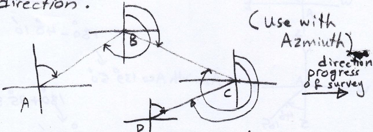
$$0^{\circ} \text{ backward direction} = \text{forward direction} + 180^{\circ}$$
