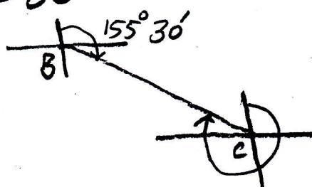
$$\begin{aligned} \text{forward } BC &= 155^\circ 30' \\ \text{backward } BC &= 180^\circ + 155^\circ 30' \\ &= 335^\circ 30' \end{aligned}$$
