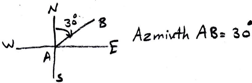
Azimuth AB =  $30^\circ$
