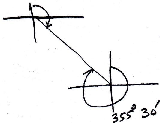
$$\begin{aligned}\text{Forward } DE &= 355^\circ 30' \\ \text{backward } DE &= 355^\circ 30' - 180^\circ \\ &= 175^\circ 30'\end{aligned}$$
