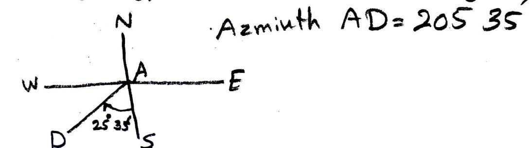
Azimuth AD =  $205^\circ 35'$
