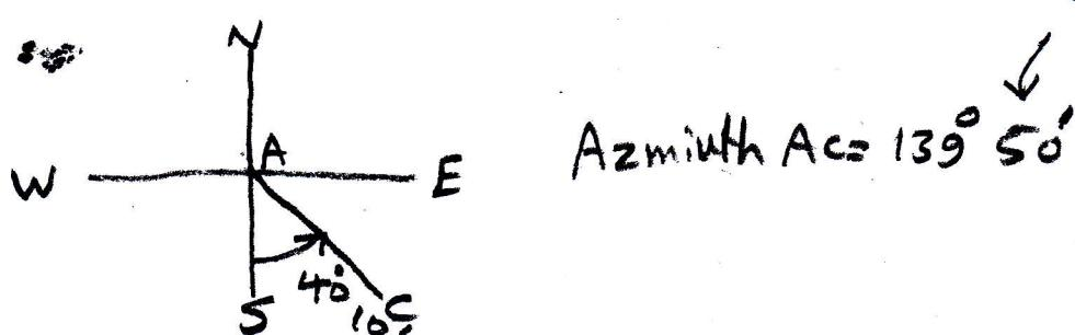
Azimuth AC =  $139^\circ 50'$
