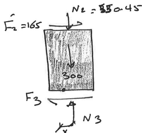
S.6 A weighs 50 N.  $\mu = 0.5$  between A and the plane, BC weighs 100 N. Determine the forces acting on body A.
