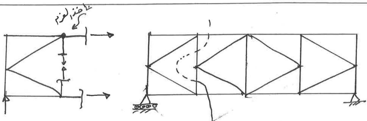
**Ex:-** For the truss shown in fig. Determine the force in member EC, BC, EB and AB
