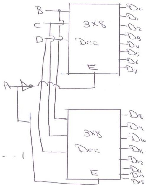
H.W:- Design 4-to-16 Decoder, Using 2x4 Decoders with enable-
