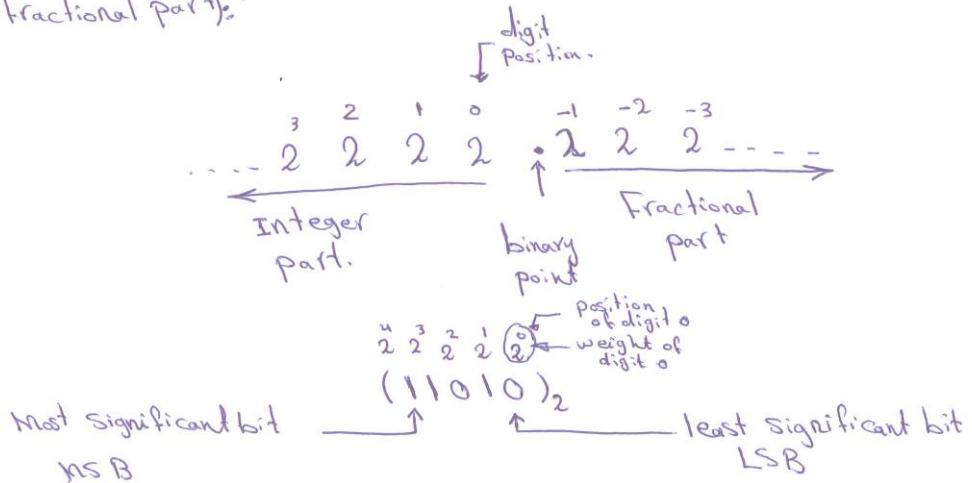
$$\begin{aligned} \text{Value} &= (1 \times 2^4) + (1 \times 2^3) + (0 \times 2^2) + (1 \times 2^1) + (0 \times 2^0) \\ &= (1 \times 16) + (1 \times 8) + (0 \times 4) + (1 \times 2) + (0 \times 1) \end{aligned}$$
