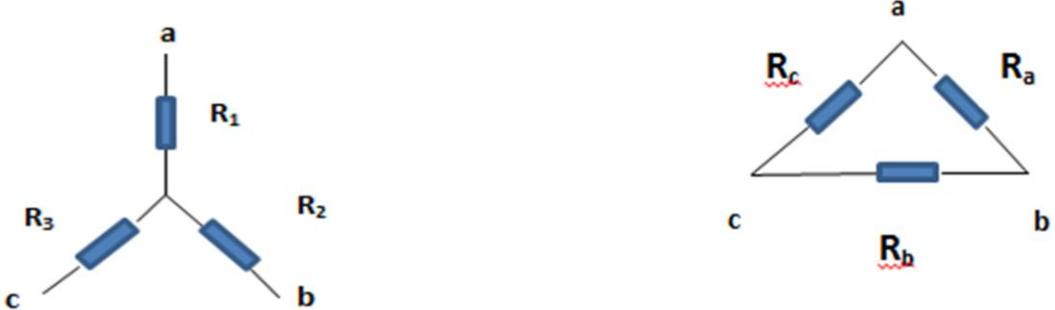
$R_{ab}$  for Star =  $R_{ab}$  for  $\triangle$
