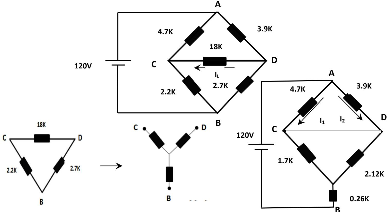
$$R_1 = \frac{18 * 2.2}{18 + 2.2 + 2.7} = 173K\Omega ; \quad R_2 = \frac{18 * 2.7}{18 + 2.2 + 2.7} = 2.12K\Omega ; \quad R_3 = \frac{2.2 * 2.7}{18 + 2.2 + 2.7} = 0.26K\Omega$$
