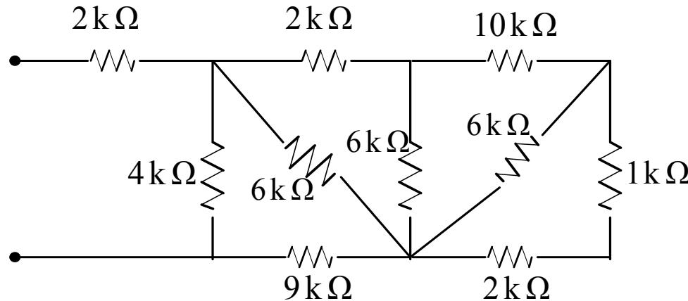
$$R_1 = \{[(1\text{k}\Omega) + (2\text{k}\Omega)] \parallel 6\text{k}\Omega\} + 10\text{k}\Omega$$
