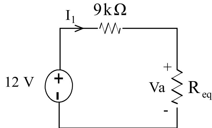
$$\begin{aligned} R_{eq} &= [(3k + 9k) // 4k] + 3k \\ &= 3k\Omega \end{aligned}$$
