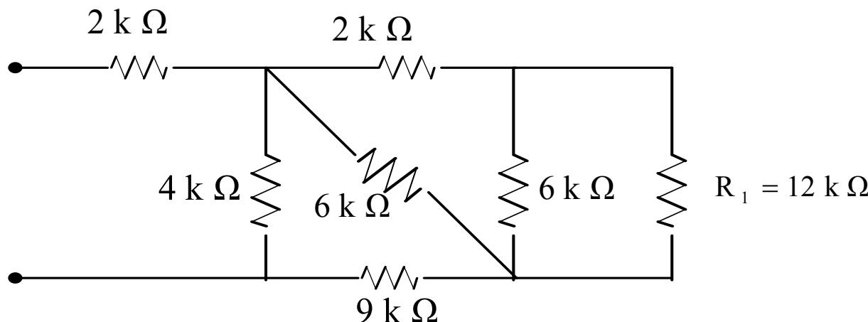
$$R2 = [12\text{k} // 6\text{k}] + 2\text{k} = 6\text{k}$$
