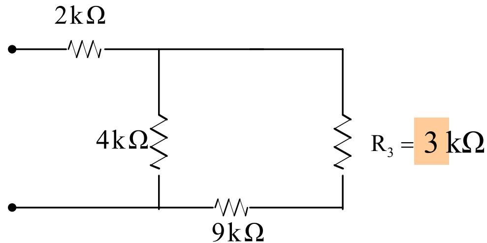
$$R_{eq} = (12\text{ k} \parallel 4\text{ k}) + 2\text{ k} = 5\text{ k}$$
