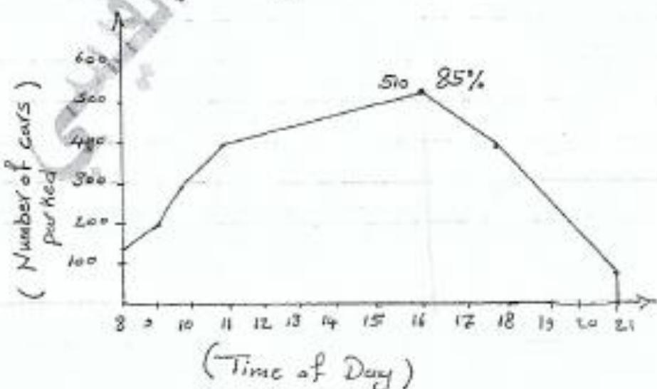
4. The parking load: The area under the accumulation curve between two specific times. It is usually given as the number of space-hours used during the specified period of time.
