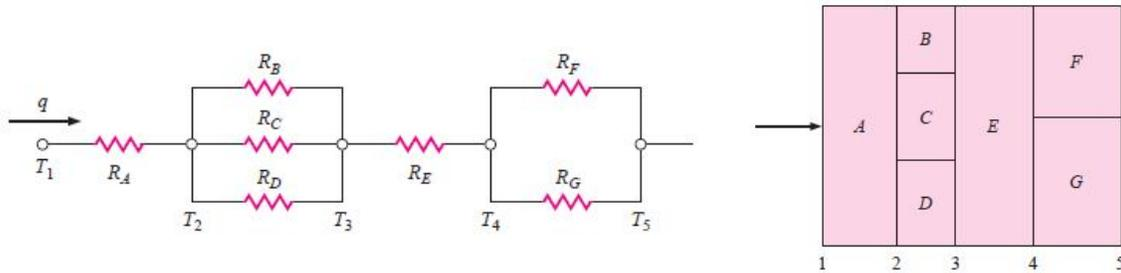
$$\frac{1}{R_1} = \frac{1}{R_A}; \quad \frac{1}{R_2} = \frac{1}{R_B} + \frac{1}{R_C} + \frac{1}{R_D}; \quad \frac{1}{R_3} = \frac{1}{R_E}; \quad \frac{1}{R_4} = \frac{1}{R_F} + \frac{1}{R_G}$$
