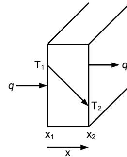
$$\text{Flow} = \frac{\text{potential (Driving Force)}}{\text{Resistance}}$$
