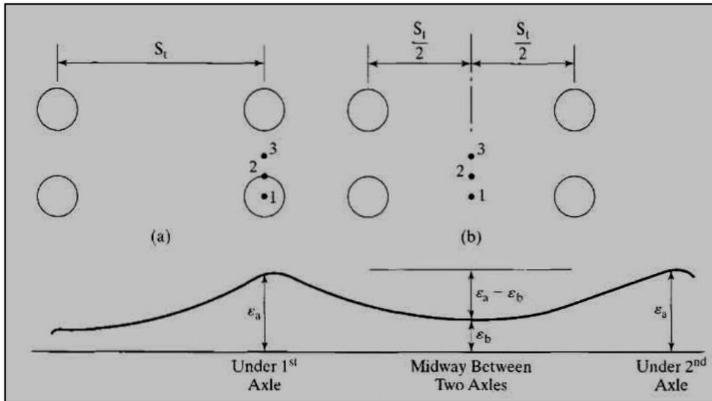
**Figure (21): Damage Analysis of Tandem-Axle Loads**
