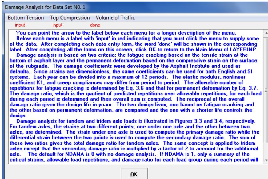
Figure (20): Damage Screen
