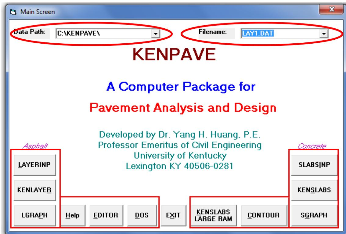
Figure (4): Details for Main Screen of KENPAVE Software
