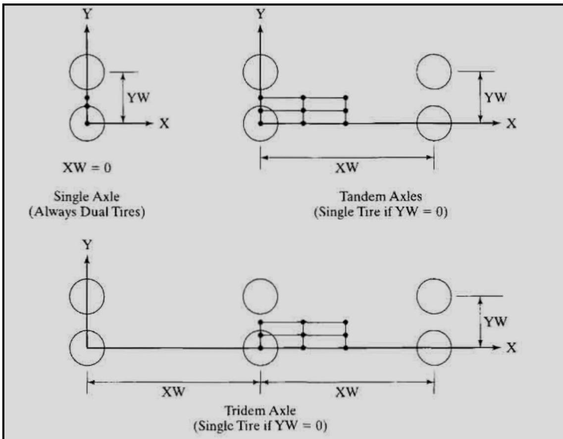
**Figure (13): Wheel and Axle Arrangements.**
