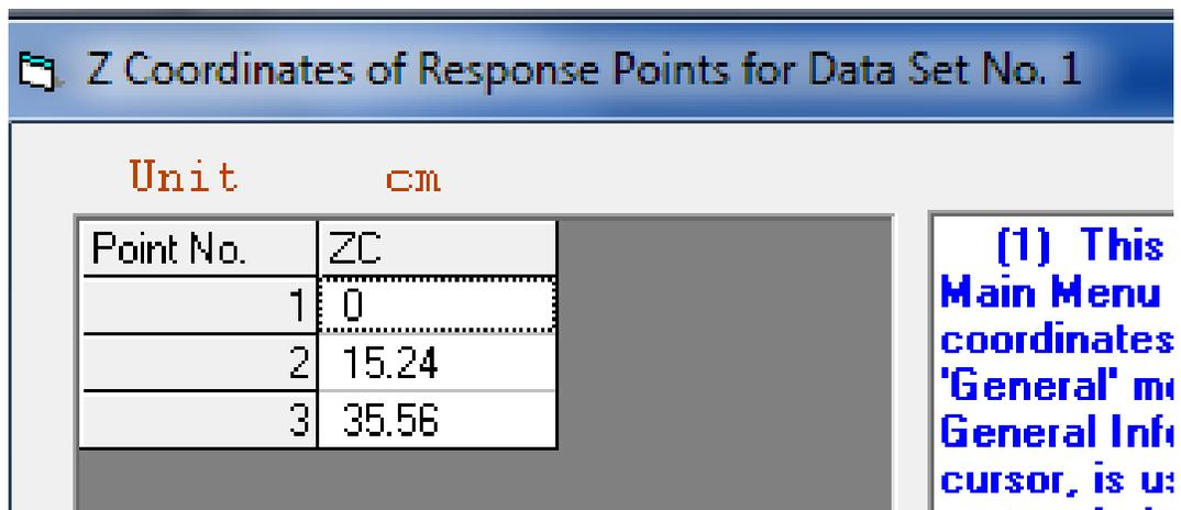
**ZC:** Enter the depth at which you want to obtain deflection output. *When the point is located exactly at the interface between two layers, the results are for the bottom of upper layer. If the results at the top of next lower layer are desired, a slightly larger z coordinate, say 0.0001 larger, should be used.*
