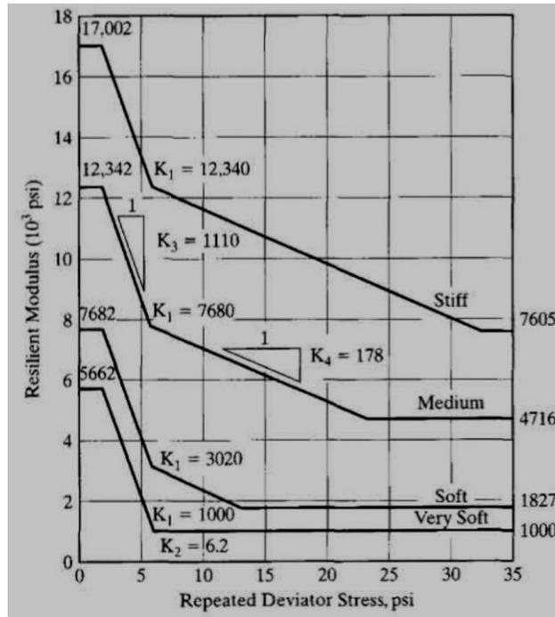
**Figure (17): Resilient-Modulus–Deviator-Stress Relationship for Four Types of Subgrade.**
