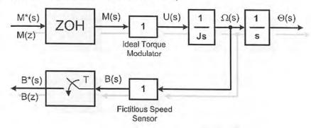
$$\begin{split} \frac{\Omega(z)}{M(z)} &= Z \Biggl\{ \underbrace{\frac{(1-z^{-1})}{s}}_{ZOH} \cdot \underbrace{\frac{1}{J} \cdot \frac{1}{s}}_{\text{Process}} \Biggr\} = \frac{1}{J} (1-z^{-1}) Z \Biggl\{ \frac{1}{s^2} \Biggr\} \\ &= \frac{\Theta(z)}{M(z)} = \frac{T}{J} \underbrace{(1-z^{-1})}_{(1-z^{-1})^2} \end{split}$$
