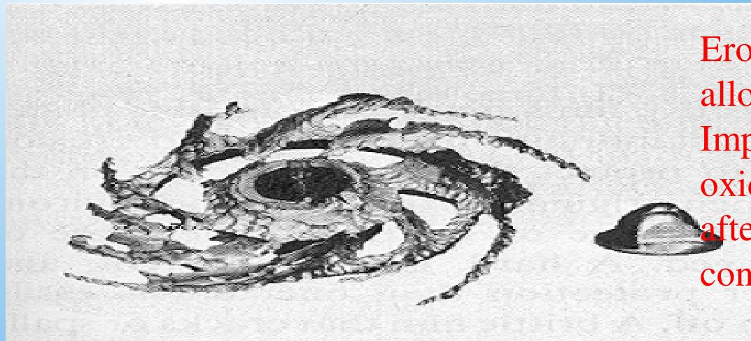
Erosion-corrosion of stainless alloy pump impeller.
