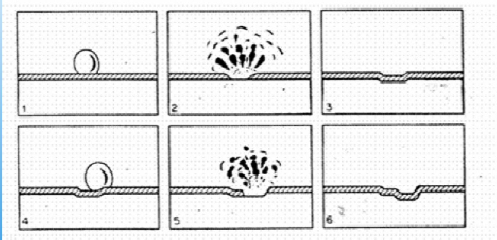
**High-speed pressure oscillations (pumps, etc.) can create shock waves  $> 60,000$  psi. Surface attack often resembles closely-spaced pitting.**
