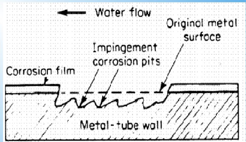
Erosion-corrosion of condenser tube wall.
