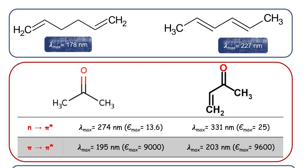
MORE conjugated double bonds MEANS LESS (E) is required for the electronic transition, and therefore LONGER  $\lambda$  at which the electronic transition occurs.
