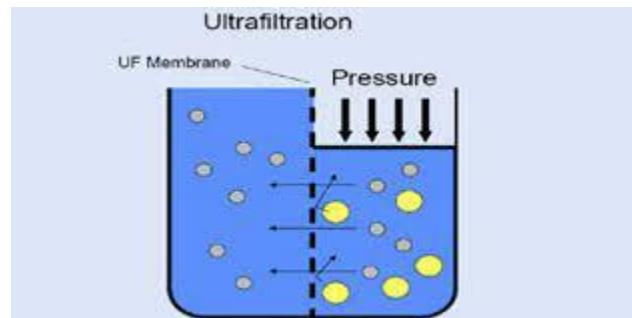
The selectivity and retentivity of a membrane are characterized by its molecular weight cut off. It is difficult to characterize the porosity of an ultrafiltration membrane by means of precise molecular weight cut off. The configuration of the molecule and its electrical charge may also affect the separation properties of the membrane
