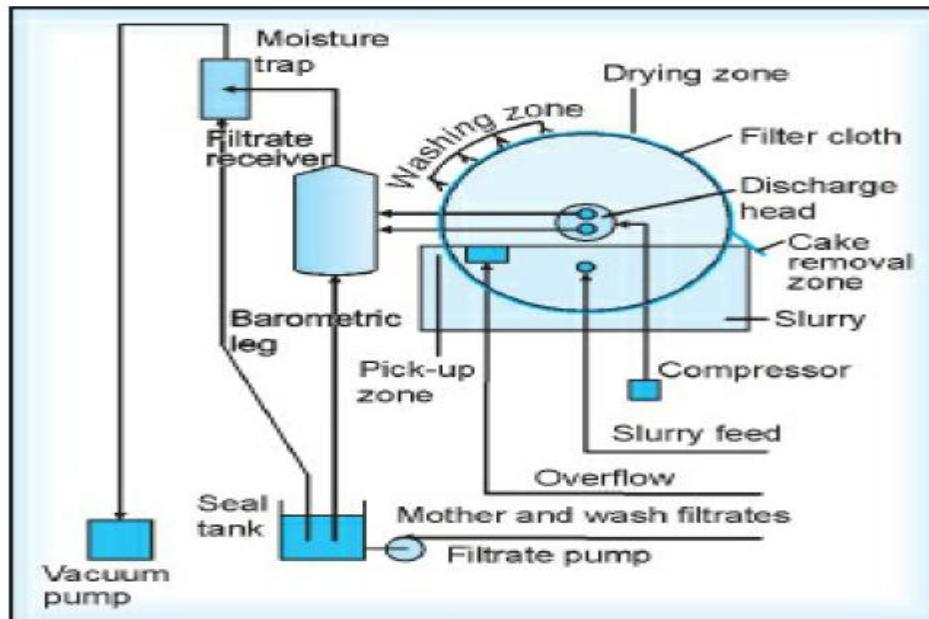
Each filter unit is rectangular in shape with a curved profile so that a number can be joined up to form a drum. Each unit has a perforated metal surface and is covered with filter cloth
