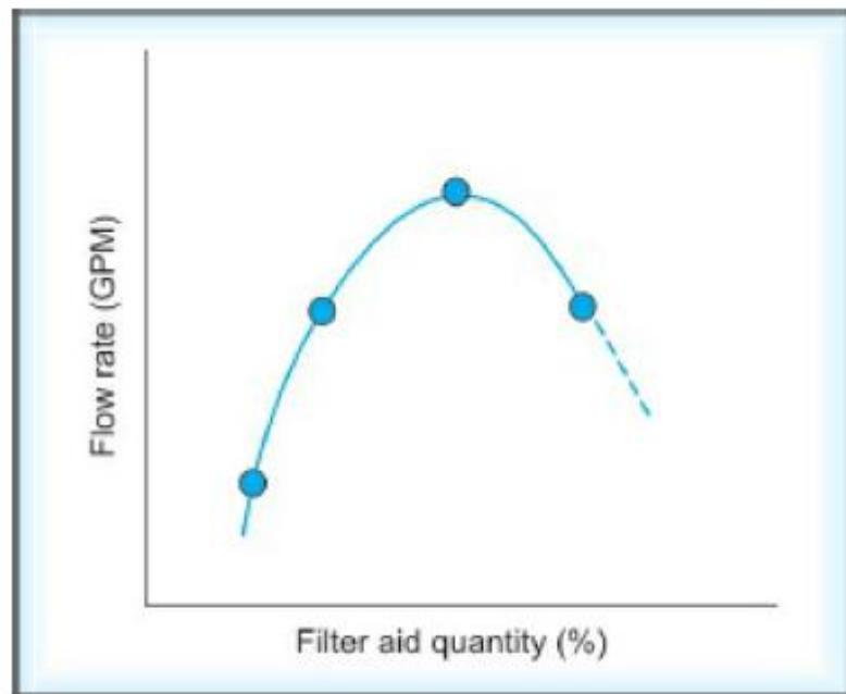
typical plot of filter aid concentration versus permeability. In the figure, flow rate and permeability are directly proportional to each other. At low concentrations of filter aid, the flow rate is low because of low permeability. As the filter aid concentration increases, the flow rate increases and peaks off. Beyond this point, the flow rate decreases as the filter aid concentration is increased
