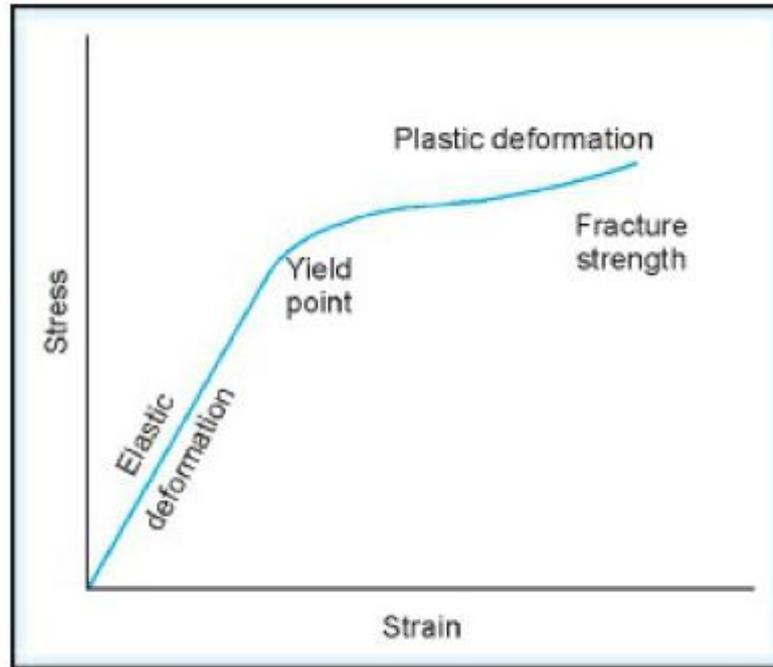
**Fig. 2.1:** Stress-strain diagram for a solid
