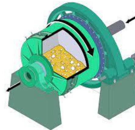
The factor of greatest importance in the operation of the ball mill is the speed of rotation.
