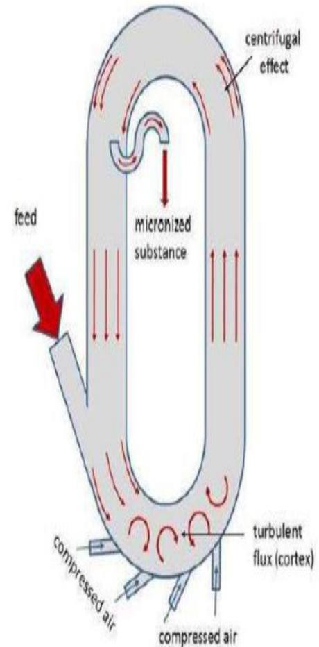
The most important machine-related factors are the grinding chamber geometry and the number and angle of the nozzles. In selecting fluid-energy mills for production, the cost of a fluid-energy source and dust collection equipment must be considered in addition to the cost of the mill
