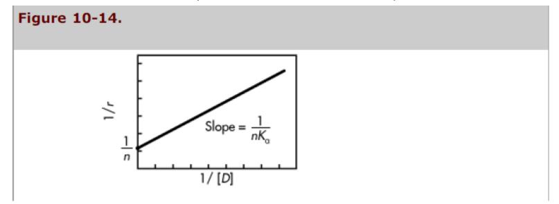
If the graph of 1/r versus 1/[D] does not yield a straight line, then the drug-protein binding process is probably more complex. Equation 10.20 assumes one type of binding site and no interaction among the binding sites.
