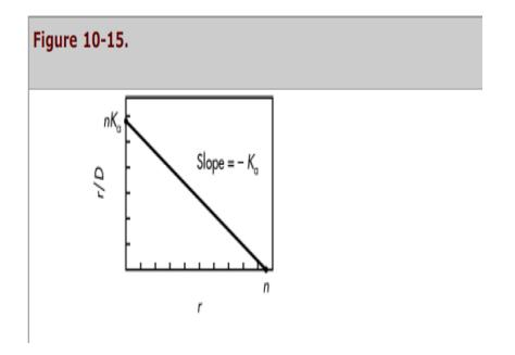
A graph constructed by plotting r/[D] versus r yields a straight line with the intercepts and slope shown in and
