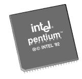
It was the miniaturisation of components and the creation of the **integrated circuit** that has made the development of modern computers possible. Although integrated circuits contain enormous numbers of components and connectors, the whole object is manufactured as a single item through special manufacturing techniques. From the outside, the integrated circuit looks like a small black box with a number of electrical connectors on the outside.
