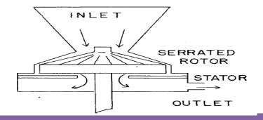
Consists of a high speed rotor & stator with conical milling surfaces between which in is an adjustable clearance.
